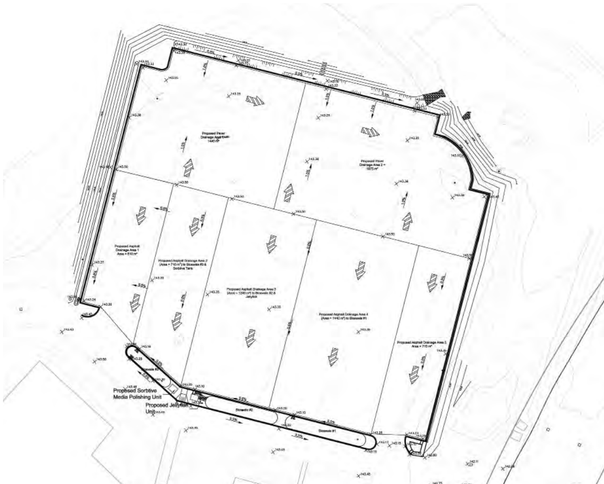
Figure 6.2.5: This proposed drainage area figure illustrates flow patterns and LID practices implemented at the IMAX Project site. Refer to the IMAX case study in Appendix A for further details. (Source: Aquafor Beech)
