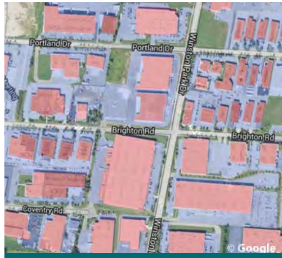
Figure 1.1.3: Commercial areas have a lot of impervious cover. This figure shows roof cover in red and asphalt cover in blue. Water can not sink into the ground so it ends up entering municipal stormwater systems or pooling on the property. (Source: CVC)
