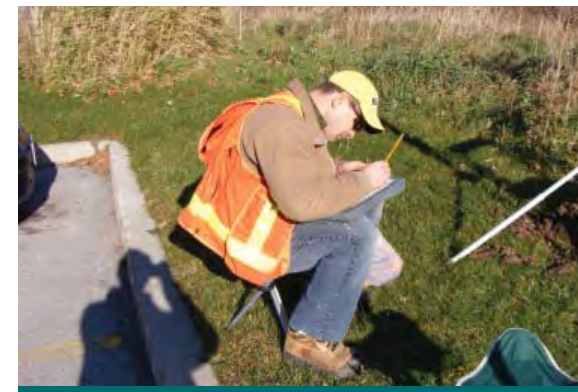
Figures 5.2.1: Fast-draining soils full of gravel and cobble will use a lot of water during testing and augering such material is difficult. Be well equipped with shovels, a sufficient water supply, and other equipment when testing. When testing clay materials, a comfortable chair is recommended. (Source: Aquafor Beech)
