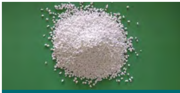
Figure 2.9.4: Photograph of an engineered phosphorus removal media. Engineered media use a variety of mechanisms to absorb and retain dissolved phosphorus. (Source: Aquafor Beech)
