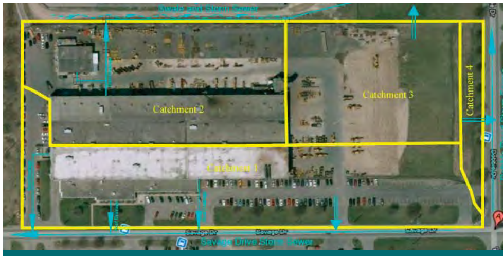
Figure 6.2.1: This figure from a stormwater management report identifies two large catchments and four roof leaders on this site. (Source: Aquafor Beech).
