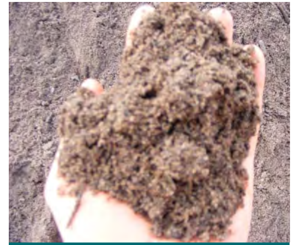
Figure 8.2.2: Mechanically mixed soil media. (Source: Aquafor Beech)
