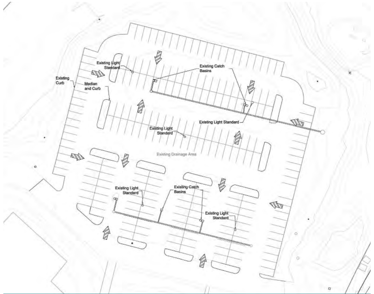
Figure 6.2.4: This pre-retrofit drainage area figure at the IMAX Project site identifies curbs, catch basins, and flow paths. Refer to the IMAX case study in Appendix A for further details. (Source: Aquafor Beech)
